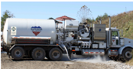
Nitrogen Pumping Unit.
